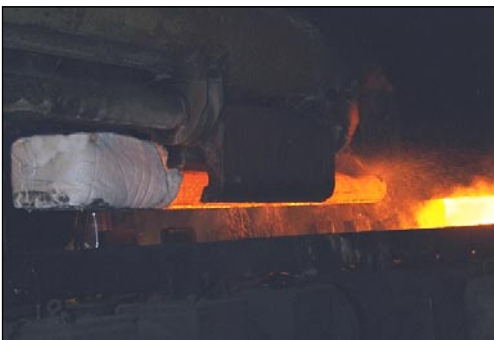
Furnace Tracker system in rotary hearth furnace
